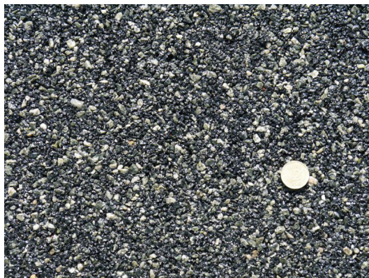
Figure 7: Poroelastic road surface. The dark particles are rubber granulates
